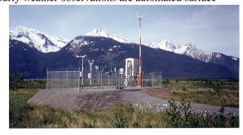
A network of **ALERT** (Automated Local Evaluation in Real Time) equipment is used primarily for hydrological purposes, measuring rainfall and river levels, but also temperature and wind in some cases. This equipment is maintained by flood control agencies in cooperation with the NWS.
