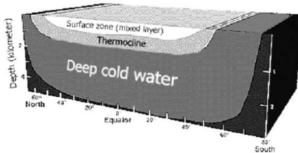
Fig. 1.06. The ocean is filled with cold water. A thin warm layer covers it, except in high latitudes. Cold and warm water are separated by a transition zone, the “thermocline.”
