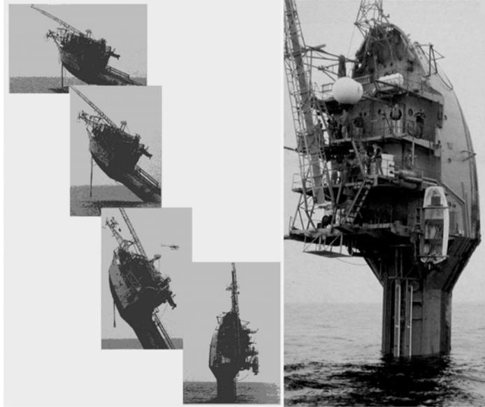
Fig. 11.09. The towed instrument platform FLIP in upright position, and ready to work.
