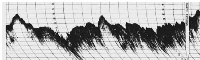
Fig. 11.04. An echo signal from the seafloor, obtained in the 1930s, by a U.S. vessel using an early type of echo recorder.
