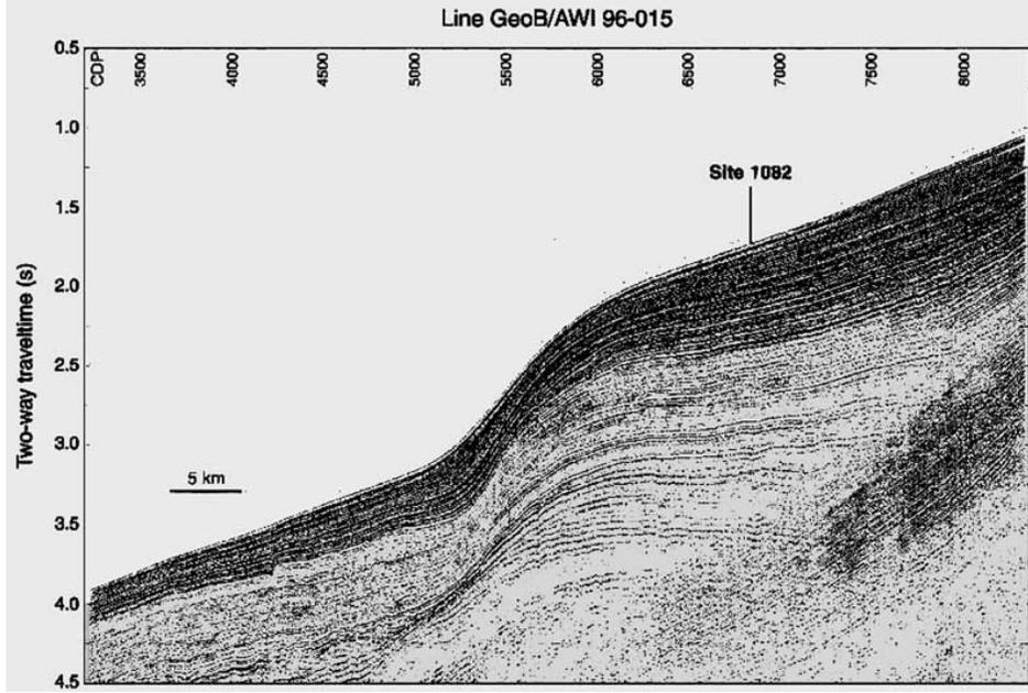
Fig. 11.13. Sediment layers on the continental slope off southwestern Africa, obtained in preparation for drilling Site 1082 of the Ocean Drilling Program, using a sound source of intermediate strength and frequency. (GeoB, Geo Bremen; AWI, Alfred-Wegener-Institut.)
