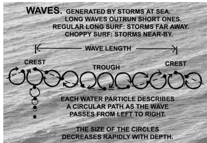
Fig. 5.08. Waves in the open ocean move energy, with water particles traveling in circles.
