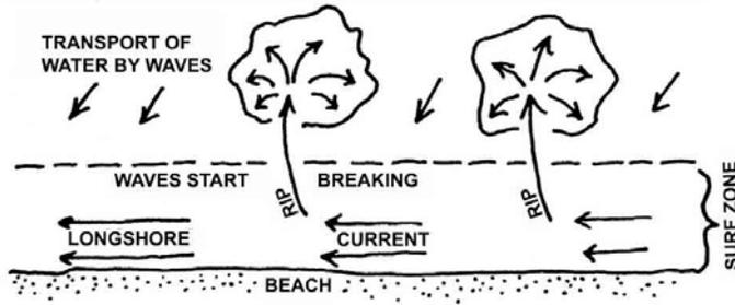
BREAKERS ARE HIGHEST ON SUBMERGED RIDGES AND ARE LOW OVER CANYONS BECAUSE OF WAVE REFRACTION: WAVES TRAVEL MORE SLOWLY OVER THE SHALLOWER AREAS AND THEREFORE BEND TOWARD SUCH AREAS.
