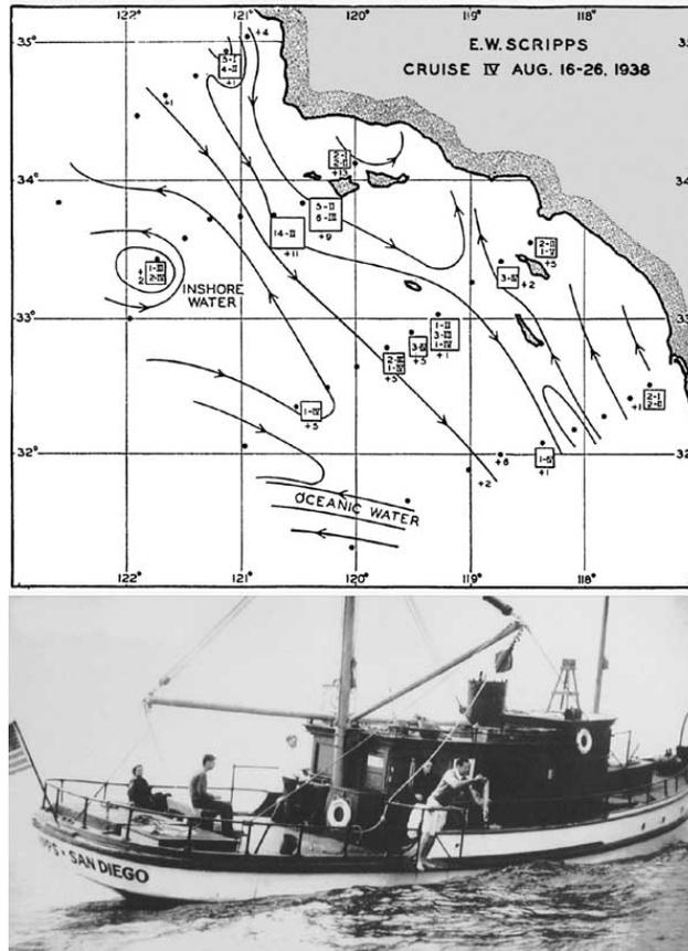
Fig. 7.07. Early results based on surveys with the motorized sailing vessel *E.W. Scripps* showed that the California Current has a complicated, ever-changing structure. Note the northward flow in the Southern California Bight.
