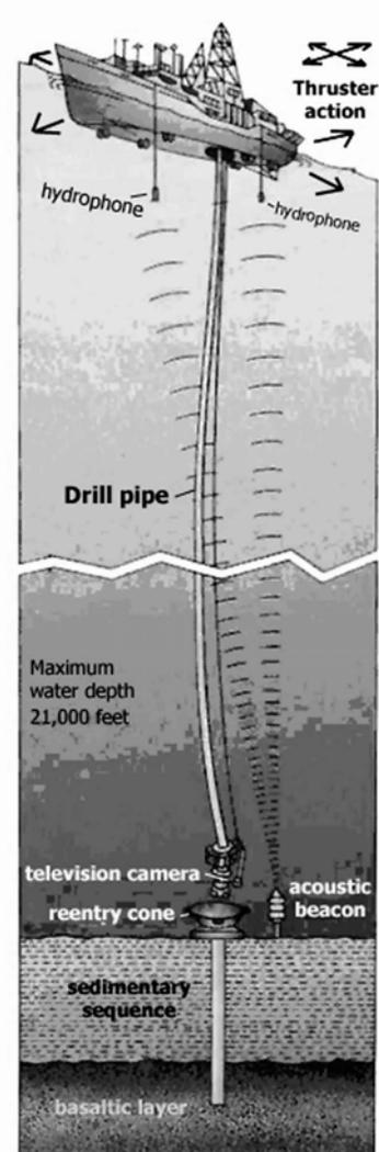
Fig. 14.01. The recovery of the memories in the deep seafloor requires modern drilling technology.
