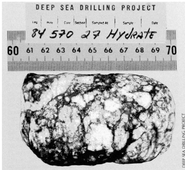
Fig. 15.09. Massive methane hydrate recovered during DSDP Leg 84, Middle America Trench. The methane is contained within a structure of water ice that is stable at high pressure and low temperature.
